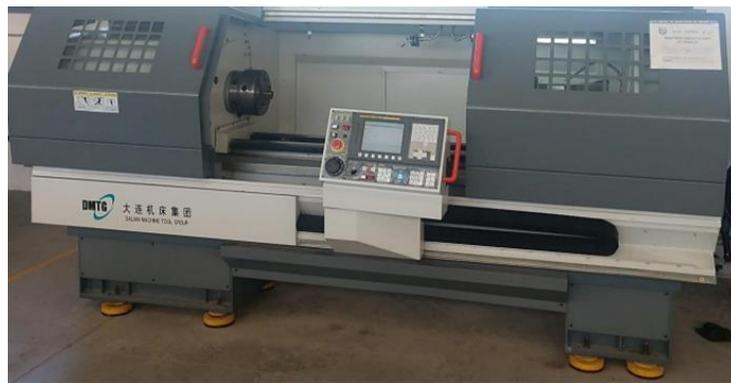
**Figura 16.** Torno CNC DMTG CKE 6150Z.
